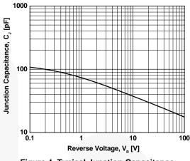
Figure 4. Typical Junction Capacitance
