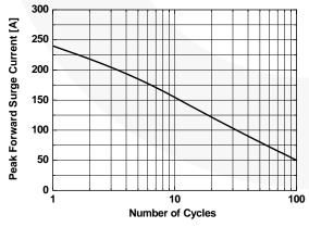
Figure 7. Maximum Non-repetitive Peak Forward Surge current
