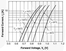
Figure 6. Typical Forward Characteristics
