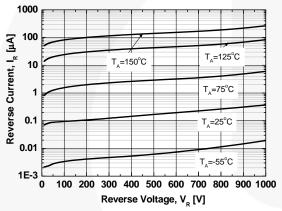
Figure 5. Typical Reverse Characteristics
