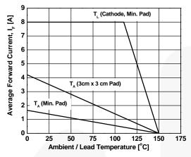
Figure 3. Forward Current Derating Curve
