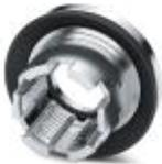
M12 threaded sleeve with tolerance-compensating function, for straight, SMD-solderable M12 socket contact inserts. Suitable for 0.9 mm ... 1.6 mm thick front plates.
