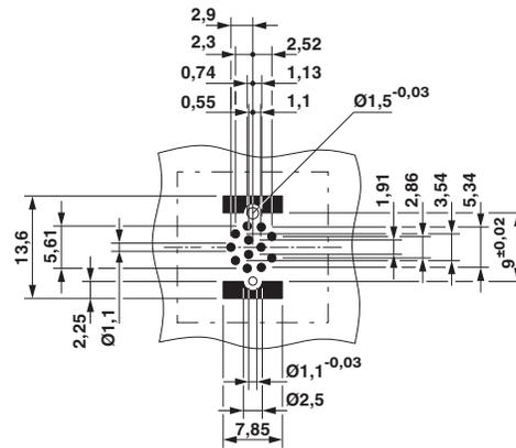
Soldering pad geometry
