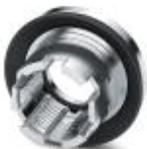
M12 threaded sleeve with tolerance-compensating function, for straight, SMD-solderable M12 socket contact inserts. Suitable for 2.3 mm ... 3.0 mm thick front plates.
