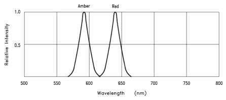
Fig.1 Relative Intensity vs. Wavelength
