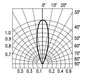
Fig.4 Relative Luminous Intensity
