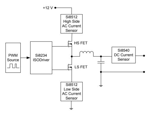
Figure 1. Open Loop POL High-Level Schematic
