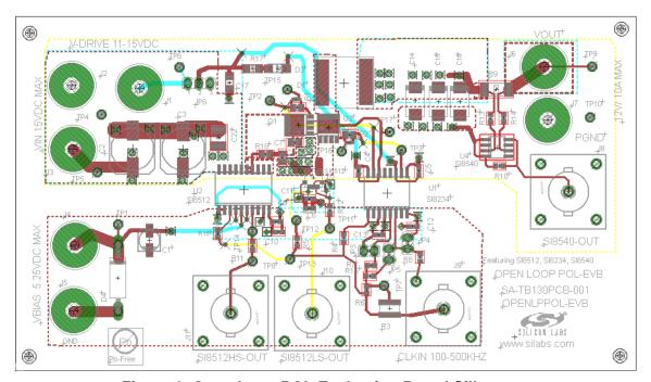
Figure 6. Open Loop POL Evaluation Board Silkscreen
