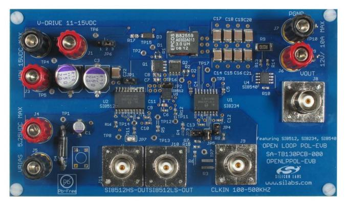
Figure 2. Open Loop POL Evaluation Board
